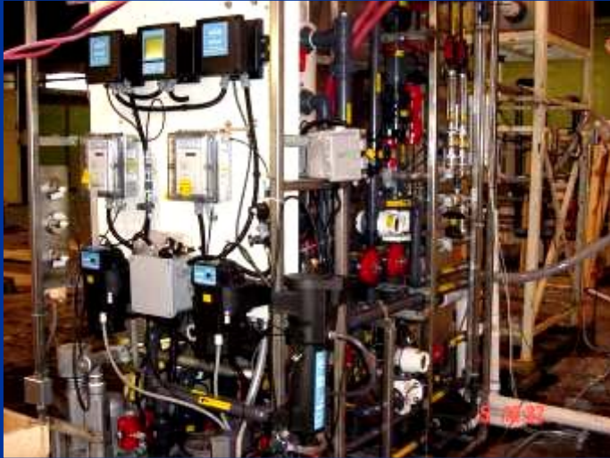
Pilot Plant – Ultra-filtration Unit
